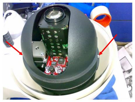
4. Remove the warranty seal and loose this screw via screw driver
